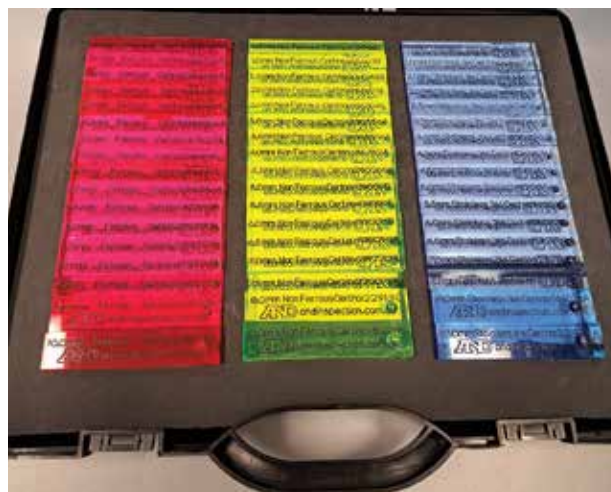
Calibration of metal detectors to recognise different metal types and size, is an important part of the detection system
