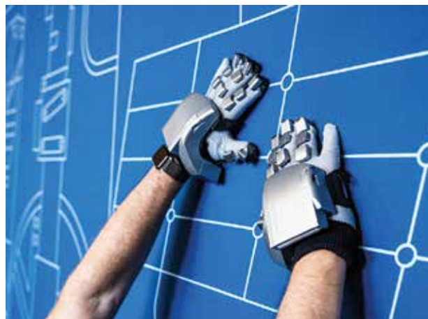
Trials are underway on a range of robotic devices to improve workers' safety including an Iron Hand to assist with grip.
