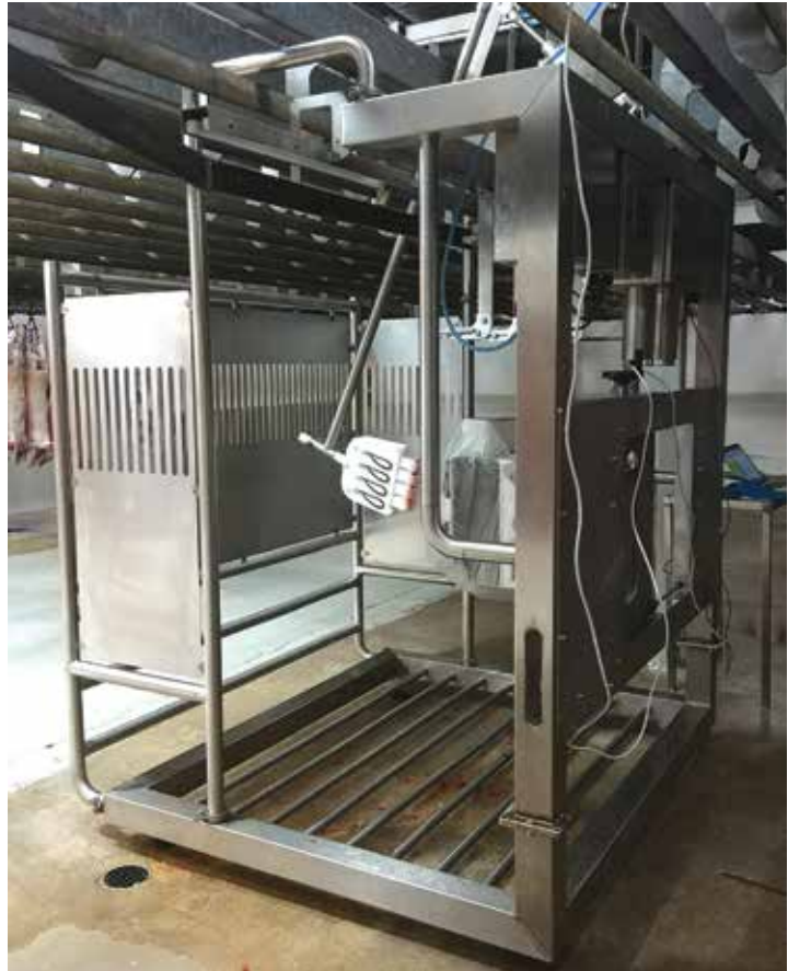
The automated sensor tool can accurately measure intramuscular fat in lamb carcasses.
