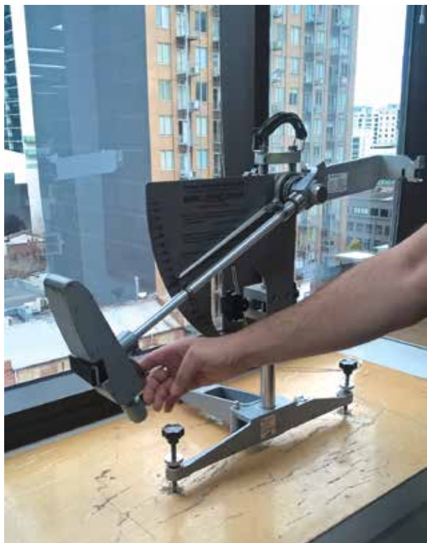
Testing of floors is performed by independent qualified laboratories using a 'pendulum' that replicates the foot-fall onto a surface.
