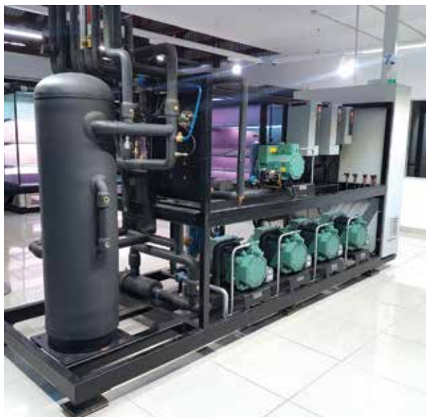
An example of a low and medium temperature rack with parallel compression (the two smaller compressors are located up high).
