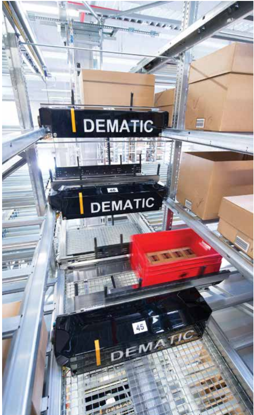
The Dematic multi-shuttle system is similar to the one installed in the NCMC Casino project. Fully automated, the cartons and SKUs are stored with full cold chain compliance and retrieved as needed, reducing OH&S issues, forklift damage and extending shelf life of products.
