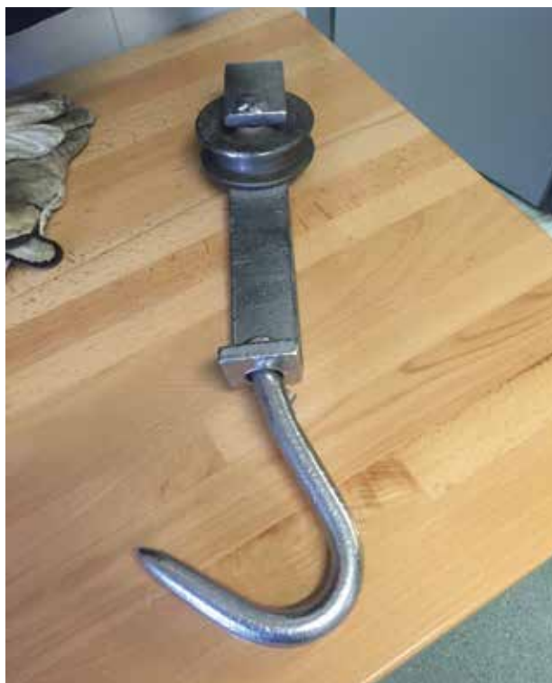
A roller book entered a rendering facility causing significant damage to plant equipment resulting in a downgrade of more than 60 tonnes of out-of-spec tallow.
